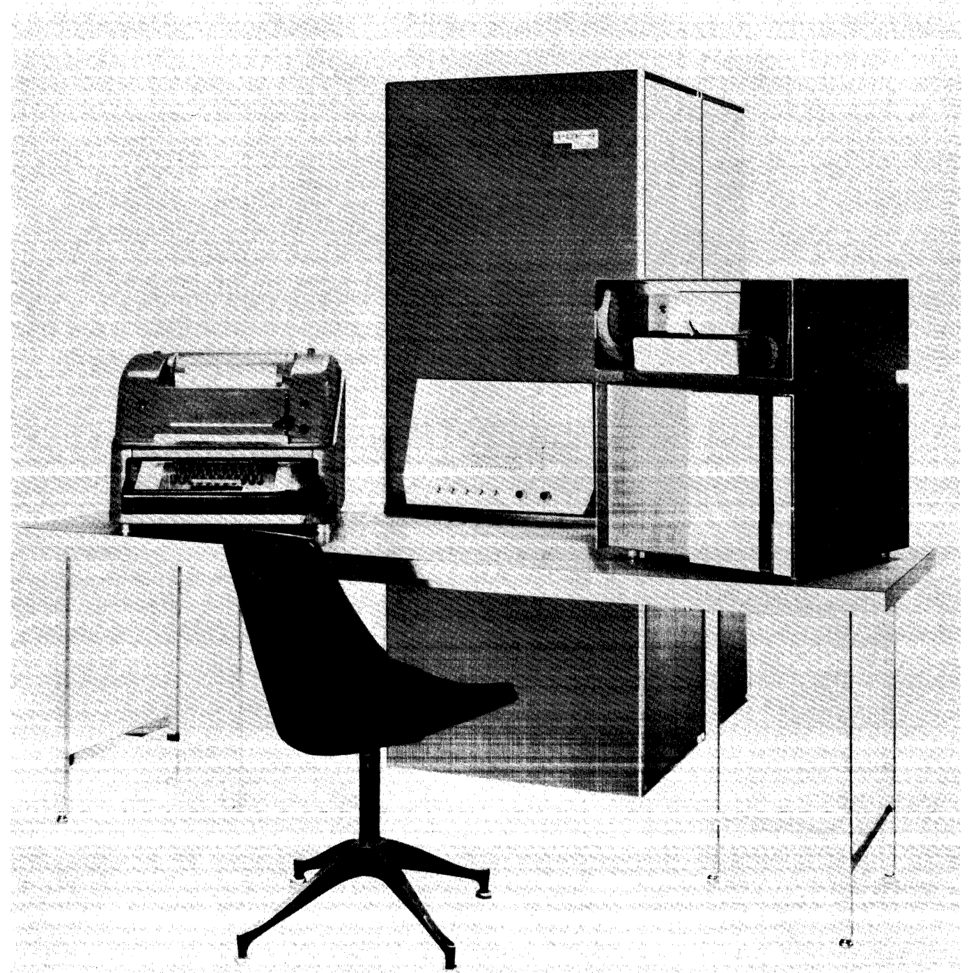
Figure 2-2 PDP-4 with Reader, Punch and Keyboard/Printer
